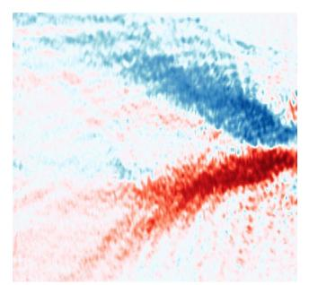
An electric field applied to a microcavity structure caused polaritons with different spins to move away from one another in opposite directions. This is visualised here by a spectrometer, with red polaritons spinning in one way separated from blue polaritons spinning the other way after they moved apart. (Image: NTU Singapore)
