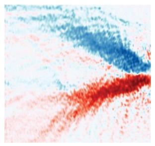
An electric field applied to a microcavity structure caused polaritons with different spins to move away from one another in opposite directions. This is visualized here by a spectrometer, with red polaritons spinning in one way separated from blue polaritons spinning the other way after they moved apart. Credit: NTU Singapore
