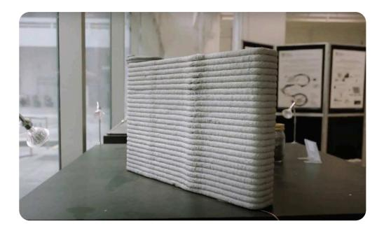
Scientists at Nanyang Technological University, Singapore (NTU Singapore) have developed a 3D concrete printing method that captures carbon, demonstrating a new pathway to reduce the environmental impact of the construction industry.
