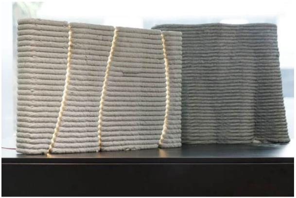
Sample of a conrete wall constructed using the newly developed 3D concrete printing method. Credit: NTU Singapore
