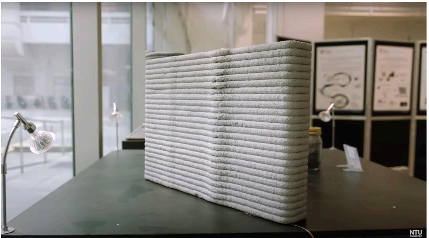
Blocks of concrete that scientists 3D-printed using a method to capture and store carbon dioxide. NTUsg / YouTube screenshot
