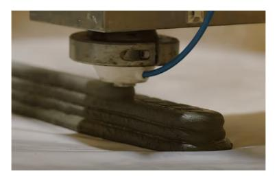
Researchers at Nanyang Technological University, Singapore, have developed a 3D concrete printing process that captures and stores carbon dioxide (CO<sub>2</sub>) during production. The method incorporates CO<sub>2</sub> and steam—by-products of industrial processes—into the concrete mix, where CO<sub>2</sub> chemically bonds into a solid form.
