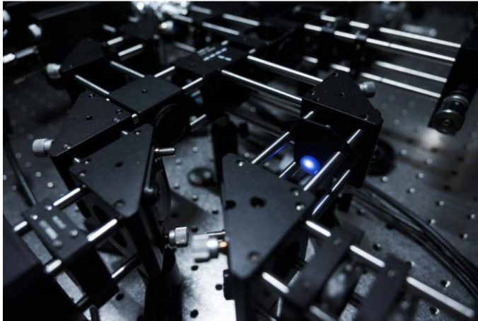
A blue laser device used to generate entangled photon pairs in an experiment at Nanyang Technological University, Singapore. Credit: Nanyang Technological University, Singapore
