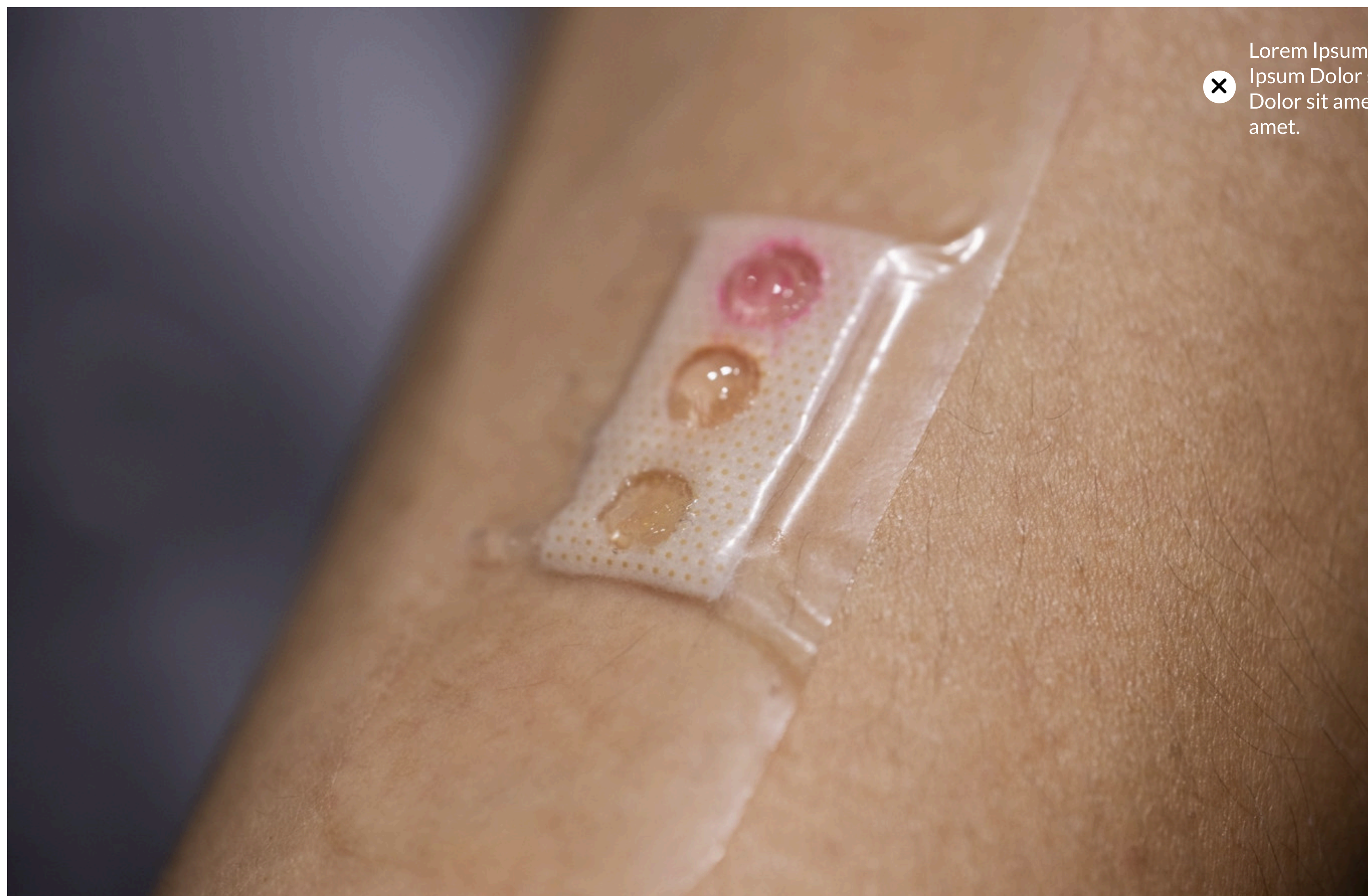
The smart plaster developed by Nanyang Technological University (NTU) Singapore researchers comprises microlaser sensors embedded in liquid crystal droplets. The sensors are customized to pick up three different types of biomarkers, namely lactate, glucose and urea. A different colored liquid crystal dot on the plaster distinguishes each biomarker. (Courtesy of NTU Singapore/)
