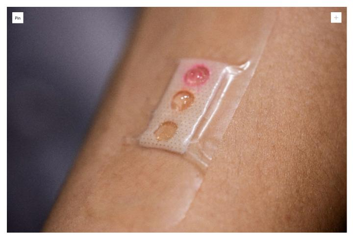
The smart plaster developed by NTU Singapore researchers comprises microlaser sensors embedded in liquid crystal droplets. The sensors are customized to pick up three different types of biomarkers (lactate, glucose, urea). A different colored liquid crystal dot on the plaster distinguishes each biomarker.
