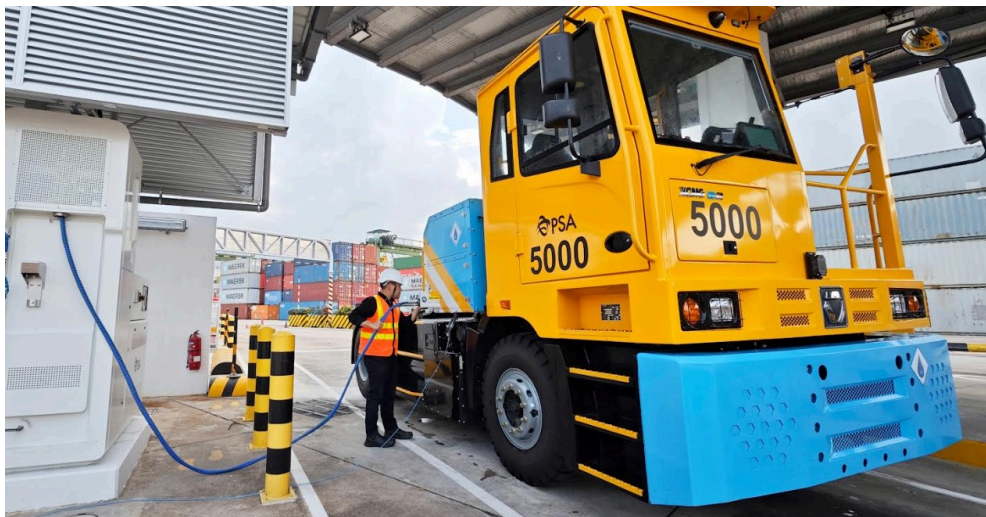
PSA Hydrogen refuelling station and fuel-cell electric prime mover
