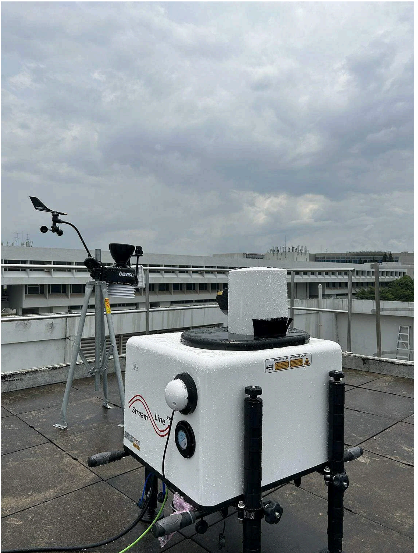
The box-like instrument can scan up to 12km of the atmosphere from the ground, but the study was limited to a scope of 3km. PHOTO: HUANG TAO, NTU
