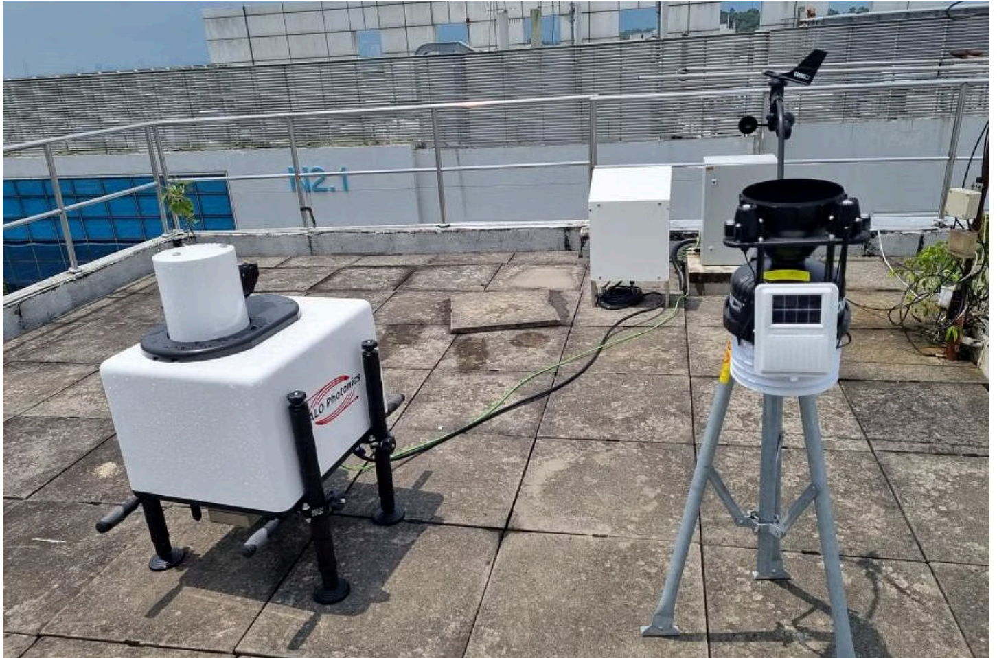
A Doppler Lidar monitoring station on the rooftop of the NTU Earth Observatory of Singapore. PHOTO: JEFFREY ENCILLO, NTU
