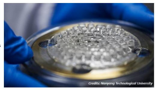
The NTU research team, led by Professor K Jimmy Hsia, found a way to maximize the adhesion of the smart adhesives by using shape-memory polymers, which can stick and detach easily when needed simply by heating them.
