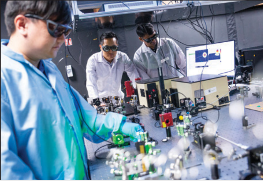
(From left) Research fellow Dr Deng Ang, Nanyang Assistant Professor Chang Wonkeun and senior research fellow Dr Trivikramarao Gavara from NTU Singapore's School of Electrical and Electronic Engineering with the experimental set-up used to generate intense and ultra-fast mid-infrared lasers. Dr Deng is calibrating the optical equipment in the set-up with a green laser.
