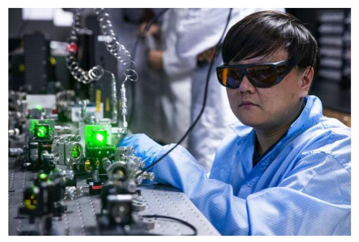
Research fellow Dr Deng Ang from NTU Singapore's School of Electrical and Electronic Engineering calibrating the optical equipment in an experimental set-up with a green laser. The set-up is used to generate intense and ultra-fast mid-infrared lasers. Credit: NTU Singapore
