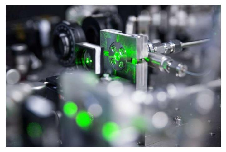
The experimental set-up used to generate intense and ultra-fast mid-infrared lasers in NTU Singapore's study. A green laser is used to calibrate the set-up's optical equipment. Credit: NTU Singapore
