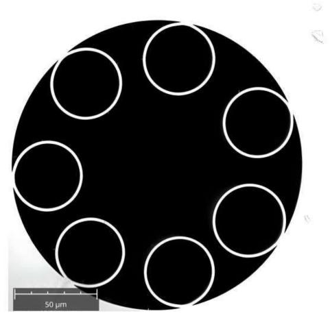
A scanning electron microscope photo of the cross-section of a hollow-core fiber used in NTU Singapore's mid-infrared laser experiments. A ring of seven smaller tubes can be seen along the inner wall of the fiber core. Credit: NTU Singapore
