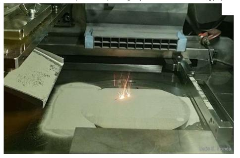
One of the laser powder bed fusion machines used in the experiments by NTU Singapore and the University of Cambridge to 3D-print metals with different properties.
