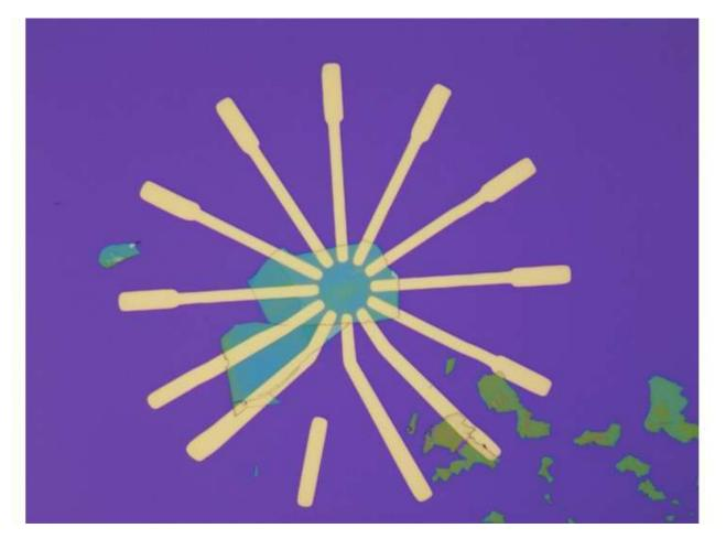
A microscopic image of the tiny device containing antiferromagnetic manganese bismuth telluride (green) that the Nanyang Technological University, Singapore researchers did their experiments on. The lines (light yellow) radiating from the center are electrodes from which current was passed through the manganese bismuth telluride. Credit: NTU Singapore
