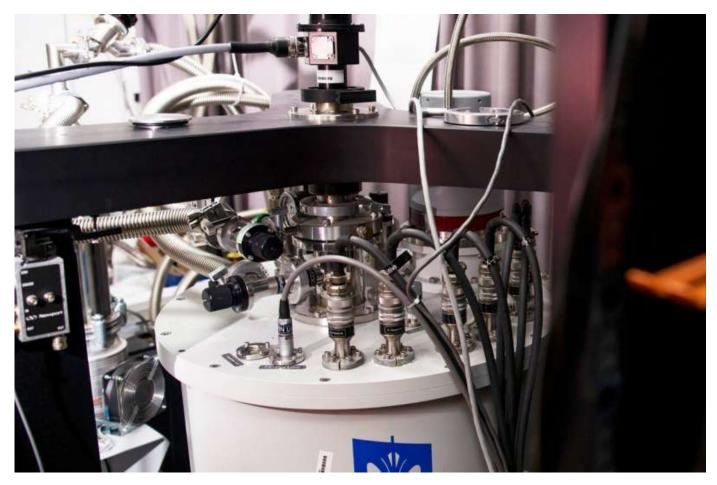
The cryogenic superconducting magnet where electrical measurements were taken in the experiments at Nanyang Technological University, Singapore. Credit: NTU Singapore
