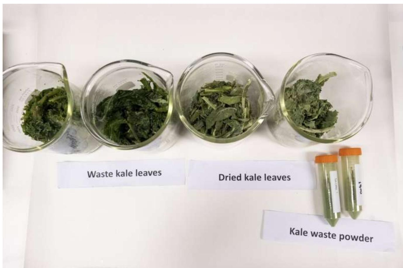
The NTU process first takes kale waste, turning it into a paste or powder form, before mixing it with a specially formulated natural deep eutectic solvent. The mixture is then filtered to extract beneficial compounds from the kale waste. Credit: Nanyang Technological University
