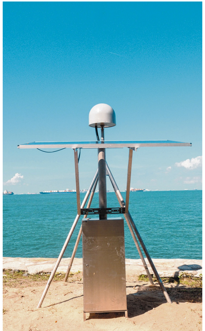
The Earth Observatory of Singapore set up the first of four reference stations on Lazarus Island in May. The stations are perched on top of tripods on a foundation of between 0.6m and 2.5m below ground for stability. PHOTO: NTU SINGAPORE/EOS
