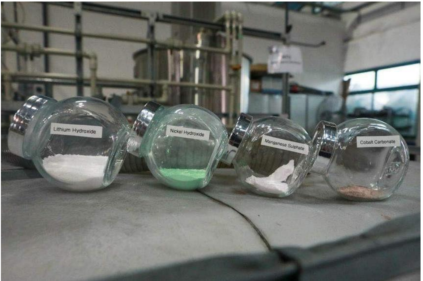
Samples of precipitated metal salts from recycling spent lithium-ion batteries at the Se-cure Waste Management recycling plant. ST PHOTO: RYAN CHIONG
