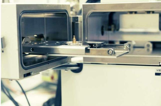
*A sample in a scanning electron microscope used in Nanyang Technological University, Singapore's quantum recoil experiments. © NTU Singapore*
