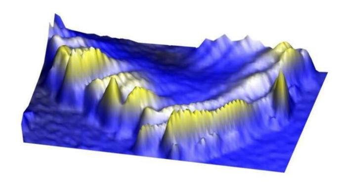
Ripples in an "electronic liquid" that were probed by the atomically sharp tip of a scanning tunnelling microscope in the researchers' experiments. Credit: SPMS/NTU Singapore
