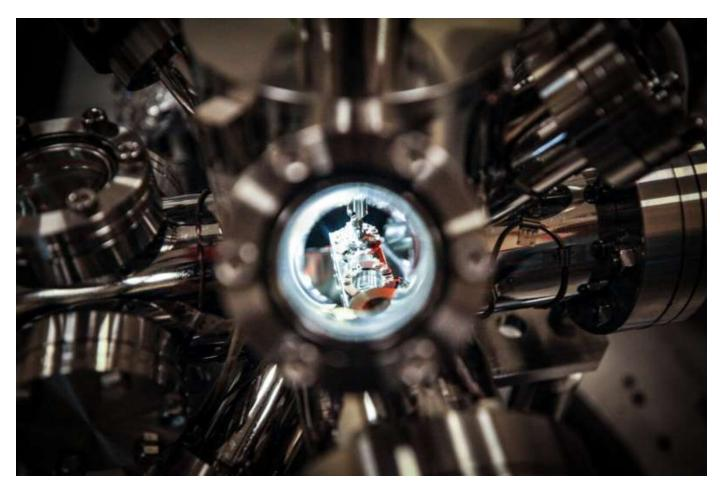
A close-up view of the tip of a scanning tunnelling microscope at NTU Singapore and a test sample inside the microscope's ultra-high vacuum chamber. The chamber is needed to reach the ultra-low temperatures for the experiments and to protect the quantum spin Hall insulators tested. Credit: SPMS/NTU Singapore
