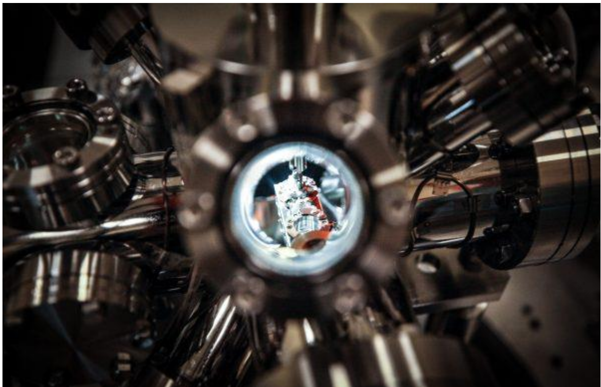
A close-up view of the tip of a scanning tunnelling microscope at NTU Singapore and a test sample inside the microscope's ultra-high vacuum chamber. The chamber is needed to reach the ultra-low temperatures for the experiments and to protect the quantum spin Hall insulators tested. Credit: SPMS/NTU Singapore.
