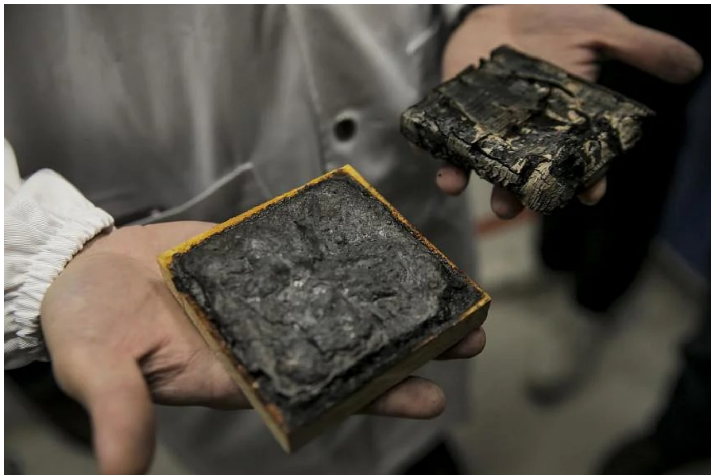
A panel of spruce wood coated with the fire-resistant resin (left) and the other without (right) after being burnt. ST PHOTO: WALLACE WOON
