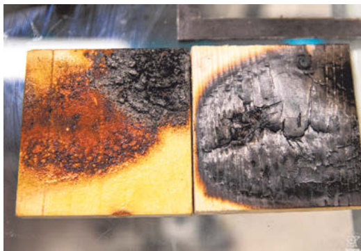
The NTU team with (above, from left) Associate Professor Aravind Dasari, Dr Sheik Anees and PhD student Dean Seah, which developed the fire-resistant resin for wood. The wood panels, one coated with a fire-resistant resin (far left) and the other without, after being burnt. ST PHOTOS: WALLACE WOON
