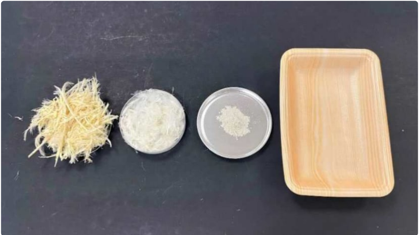
A step-by-step depiction of how chicken feathers are washed and ground into keratin powder, and the packaging materials which they would be used to manufacture. (Photo: NTU Singapore)
