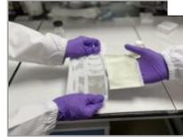
A crucial component in the fabric is a polymer that, when pressed or squeezed, converts mechanical stress into electrical energy. It is also made with stretchable spandex as a base layer and integrated with a rubber-like material to keep it strong, flexible, and waterproof.
