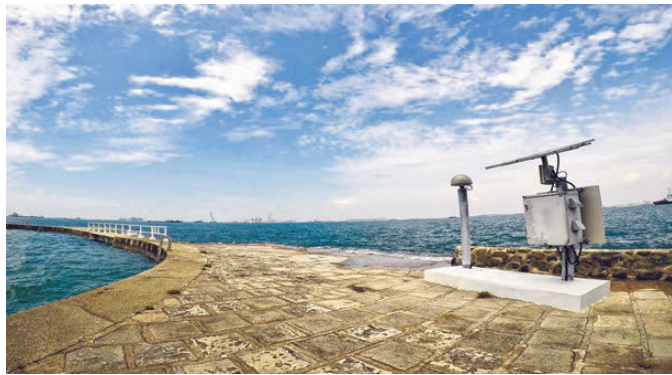
One of the Singapore Satellite Positioning Reference Network stations. Up to four new coastal global navigation satellite system reference stations will be installed across the island for data collection. PHOTO: SINGAPORE LAND AUTHORITY
