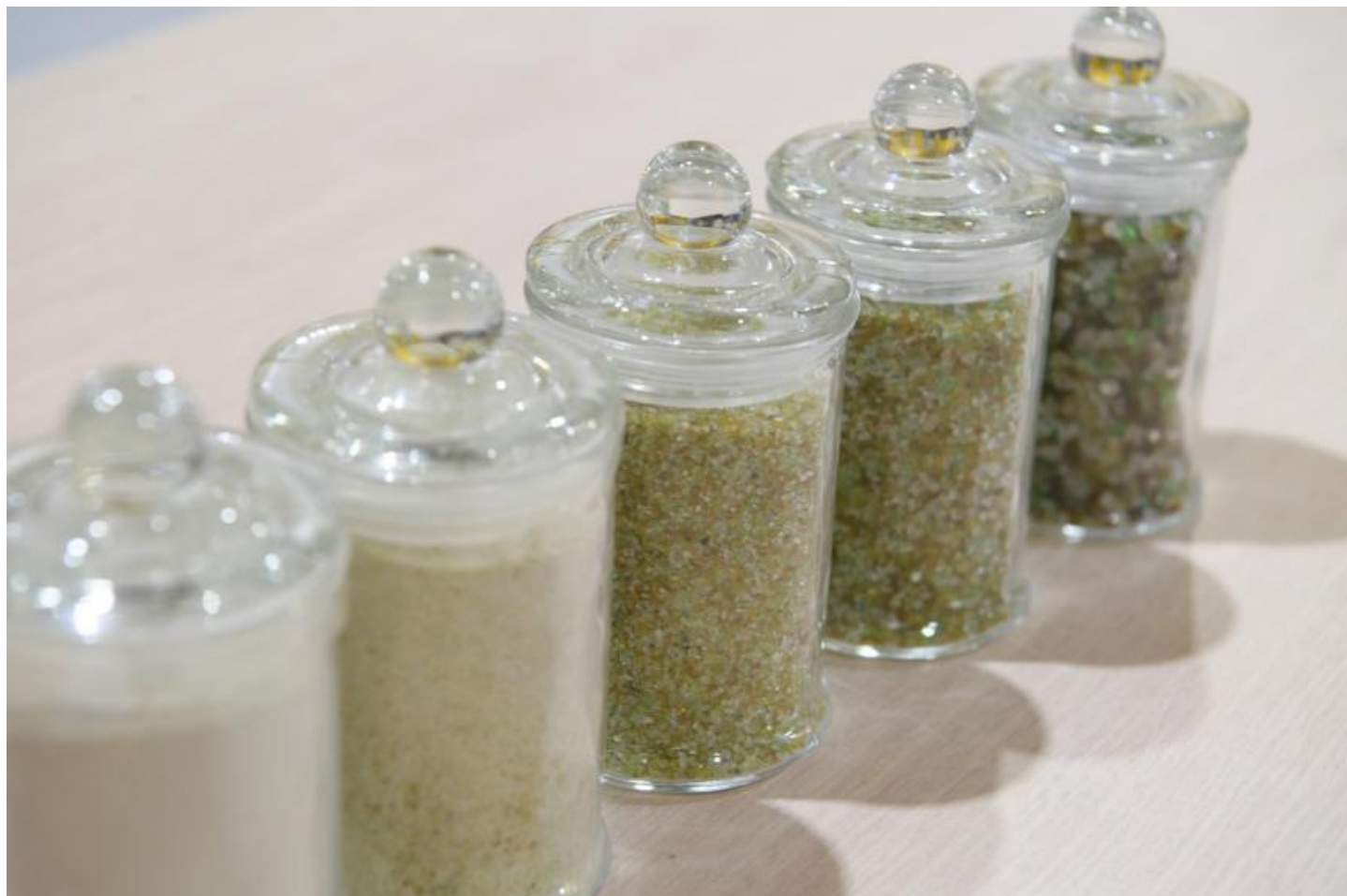
The bottles containing recycled glass are grinded down to different sizes. ST PHOTO: NG SOR LUAN
