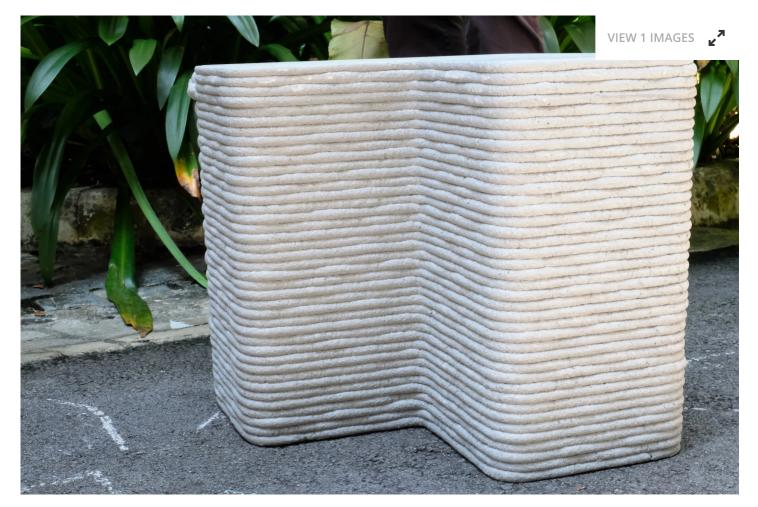
A 3D-printed bench, made of concrete in which ground glass was used in place of sand Nanyang Technological University
