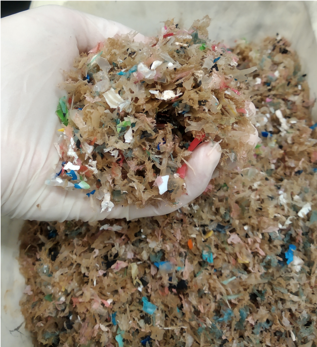
Crushed plastic litter which is then fed into the pyrolysis system for processing. Photo by NTU
