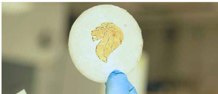
A biodegradable printed paper battery. Photo Credit: Nanyang Technological University, Singapore
