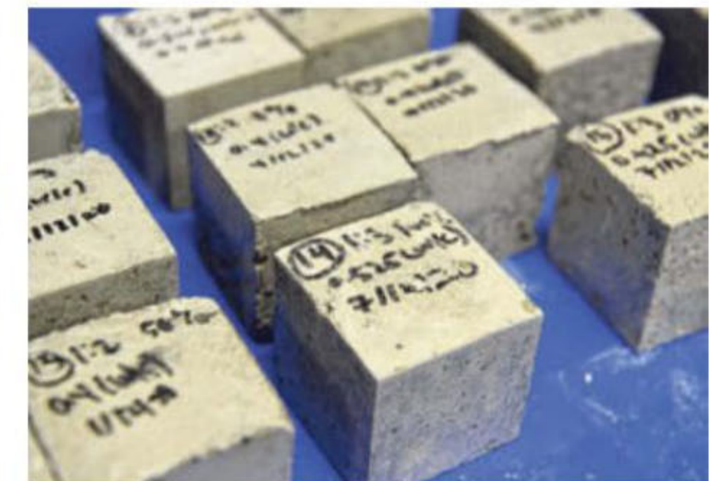
Samples of sustainable construction materials made from waste residue. Nanyang Technological University's project was one of 12 awarded a combined $55 million in grants under the national Low-Carbon Energy Research Funding Initiative, which seeks to reduce carbon dioxide emissions.
