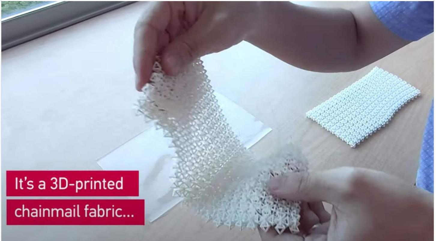
A team of researchers, including scientists from NTU Singapore and Caltech, have been working to develop a new smart fabric that is soft and flexible but can stiffen on-demand. The material is flexible like a piece of cloth yet can provide protection to the wearer when needed. It's 3D printed from a nylon polymer and consists of hollow octahedrons.
