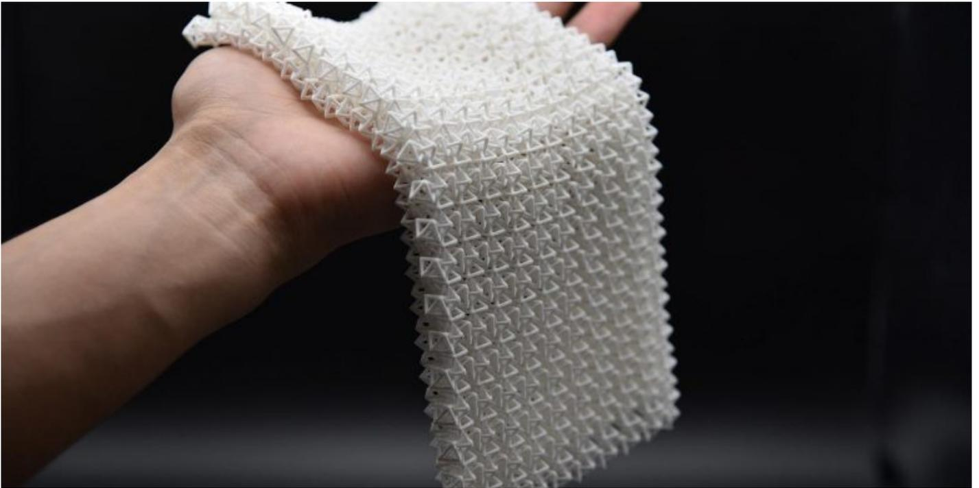
Engineers have developed a material inspired by chain mail that can transform from a foldable, fluid-like state into specific solid shapes under pressure. Credit: Caltech
