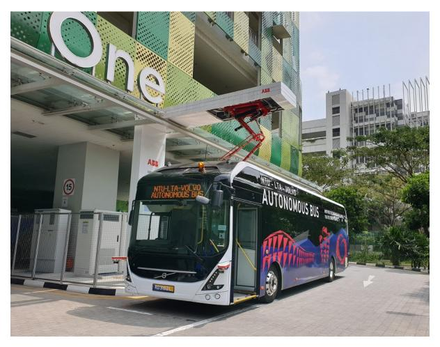
With Singapore's plans to switch its entire fleet of buses – numbering around 5,800 now – to <u>electric and hybrid buses by 2040</u>, fast charging systems that can cater to high power output – over a few hundred times higher than those required by electric cars – will be required. Current electric vehicle chargers are relatively low powered and may take many hours to fully recharge the large capacity batteries in electric buses.
