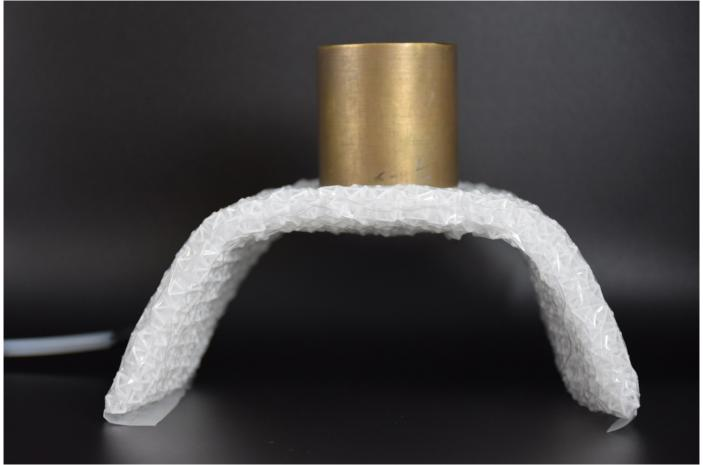
When stiffened, the new chain mail fabric can withstand up to 50 times its own weight. © NTU
