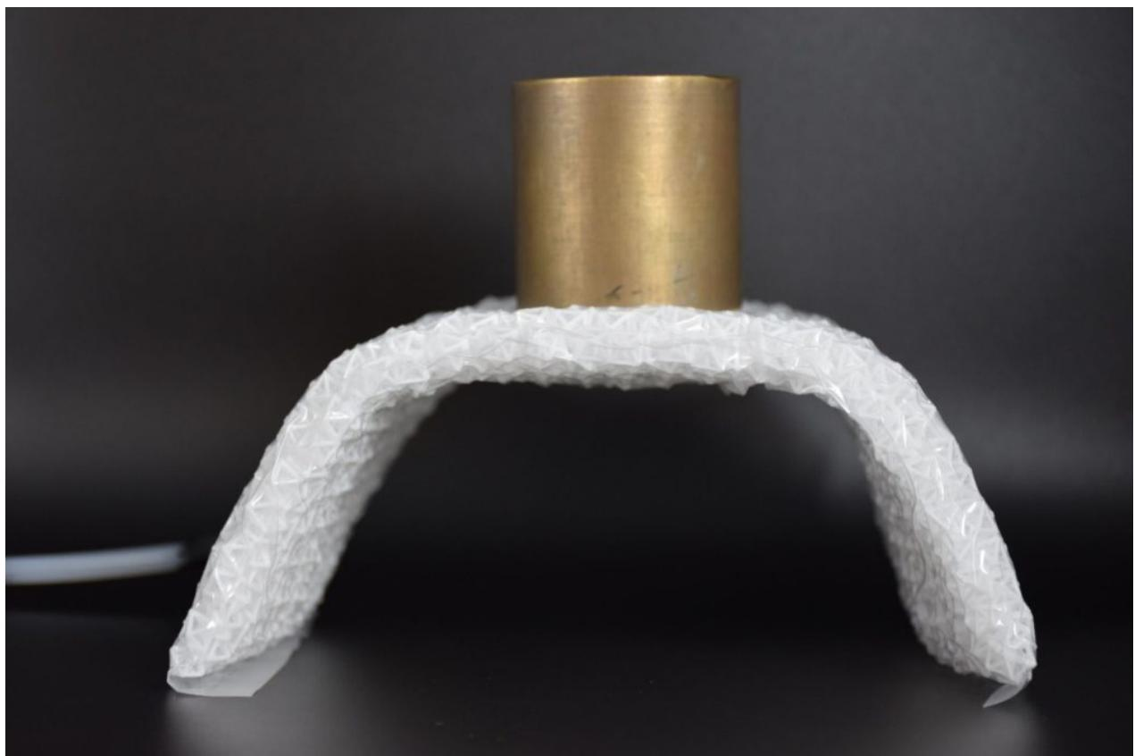
These fabrics can be 3D printed in one go on one machine and still be comprised of different interlocking shapes. The number and size of these structures, as well as the size of the fabric itself, could be changed per application. The team states that, when the hollow nylon 3D printed fabric is stiff it can hold, “1.5kgs, more than 50 times the fabrics’ own weight”. They also measured a “six times reduction in penetration depth.”
