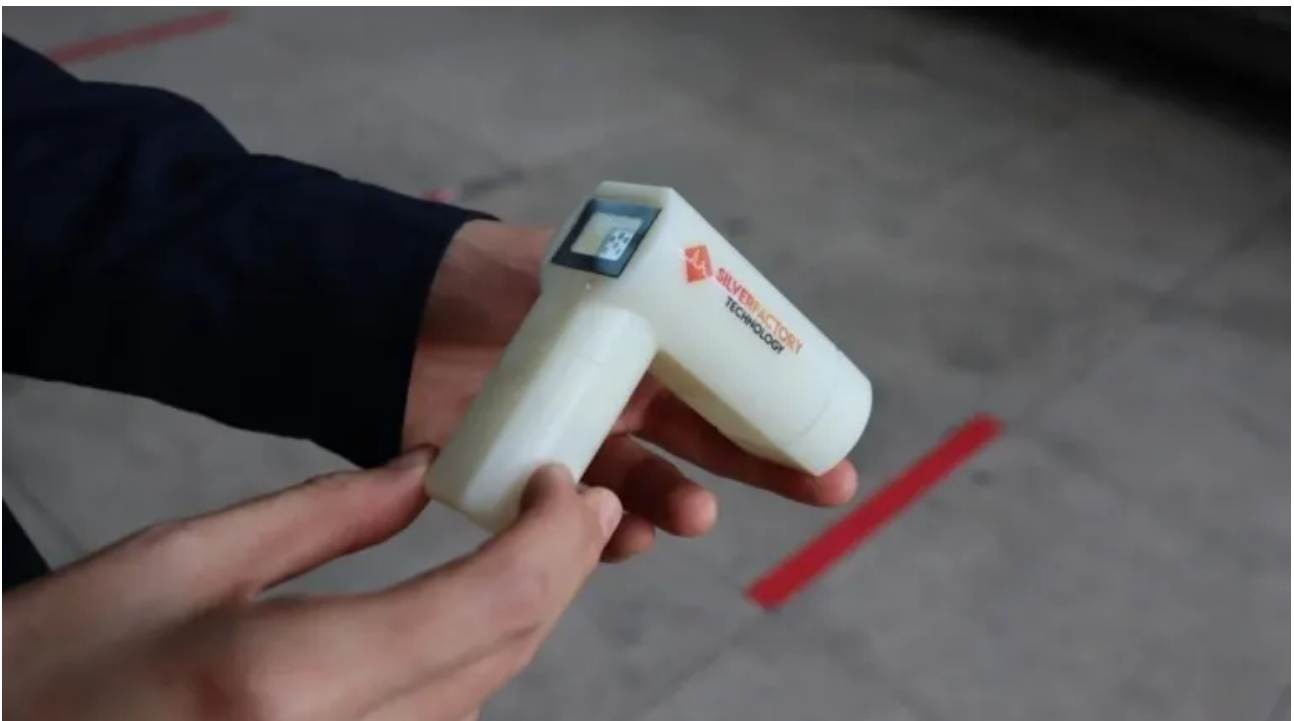
Silver Factory Technology's miniature breathalyzer can detect a coronavirus infection in 2 minutes or less. (Photo by Mayuko Tani).
