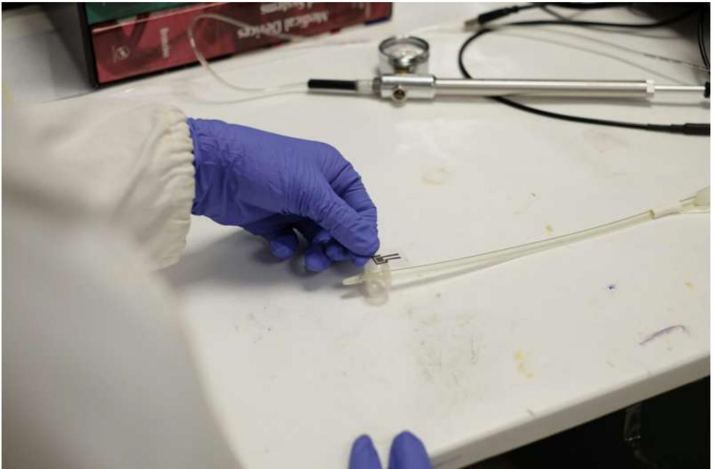
The Voltaglue patch can be applied to a deflated catheter. Once inserted into a blood vessel, the catheter can be inflated at the site of a break where the patch is activated to harden it and glue the hole shut.
