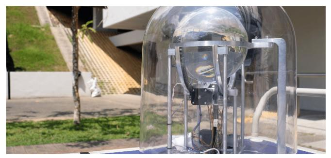
The 'smart' device includes a transparent dome-shaped cover for protection against environmental conditions | Photo source NTU Singapore
