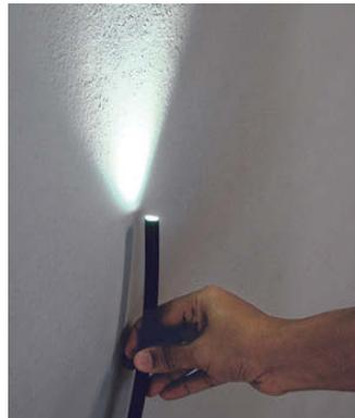
The plastic fibre cable collects and relays harvested sunlight to underground spaces. The current device developed by the researchers can relay an optimal output of sunlight up to two levels underground for optimal usage.
