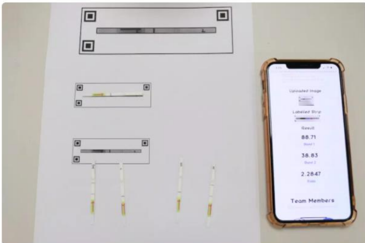
For ease of use, the scientists integrated the test into a paper test strip that can be analysed with a mobile application. Two bands appear on the strip in the presence of the SARS-CoV-2 virus. (PHOTO: Nanyang Technological University)
