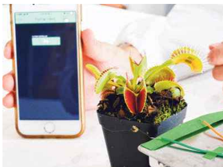
In one experiment, the team pasted a 3mm-wide electrode onto one of the traps of the Venus flytrap. Within 1.3 seconds of the smartphone sending electric pulses to the electrode, the Venus flytrap snapped shut. PHOTO: NTU SINGAPORE
