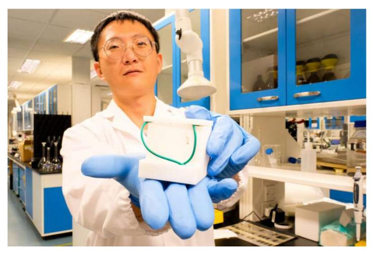
Mr Fu Xiaoxu holding up the portable skin mapping device, which weighs only 100 grams and is the size of a credit card. Credit: Nanyang Technological University
