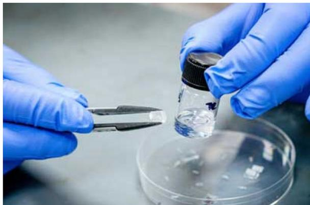
*A close up of the new piezoelectric crystal developed by NTU scientists, which can flex up to 40 times more than the conventional ferroelectric crystals typically used in small actuators and sensors. (Image: NTU)*
