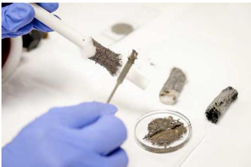
*The new magnetocuring glue is applied just like normal glue, and has a similar strength to conventional epoxy after curing. (Image: NTU Singapore)*
