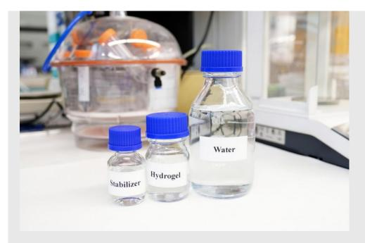
The liquid mixture used to create the smart window is made from micro-hydrogel, water, and a stabilizer. Credit: NTU Singapore
