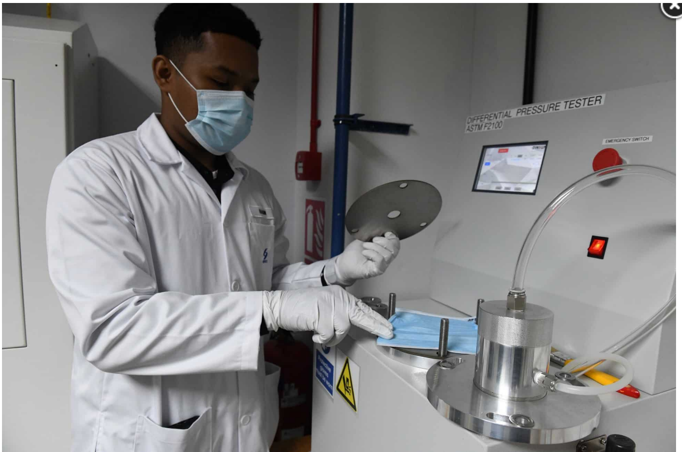
A lab technician places a face mask through a differential pressure tester during a media tour of a Setsco laboratory that tests surgical masks in Singapore. Photo: AFP/Roslan Rahman
