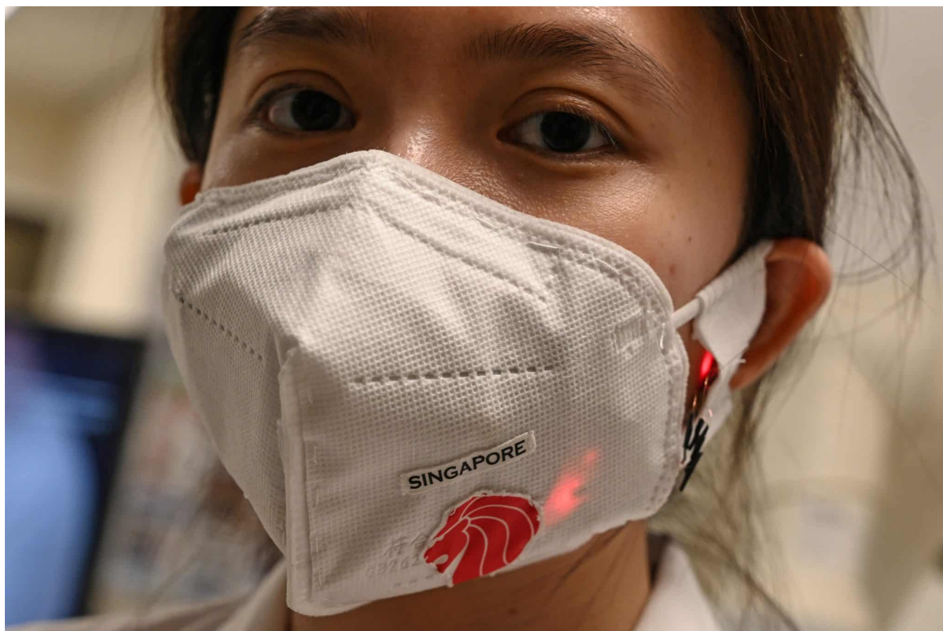
A research fellow from the School of Materials Science and Engineering at the Nanyang Technology University wearing a face mask installed with sensors which transmit via Bluetooth readings of a person’s skin temperature, blood pressure, heart rate and blood oxygen levels to a mobile application in Singapore. Photo: AFP/Roslan Rahman
