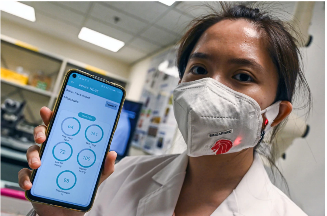
This photograph taken on September 16, 2020 shows a research fellow from the School of Materials Science and Engineering at the Nanyang Technological University wearing a face mask installed with sensors which transmit via Bluetooth readings of a person's skin temperature, blood pressure, heart rate and blood oxygen levels to a mobile application in Singapore. Roslan Rahman / AFP
