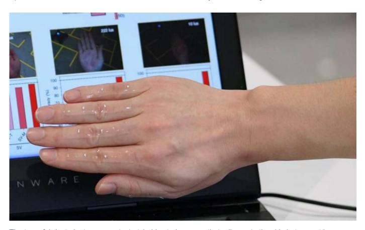
The team fabricated a transparent, stretchable strain sensor that adheres to the skin but cannot be seen in camera images. Credit: NTU Singapore
